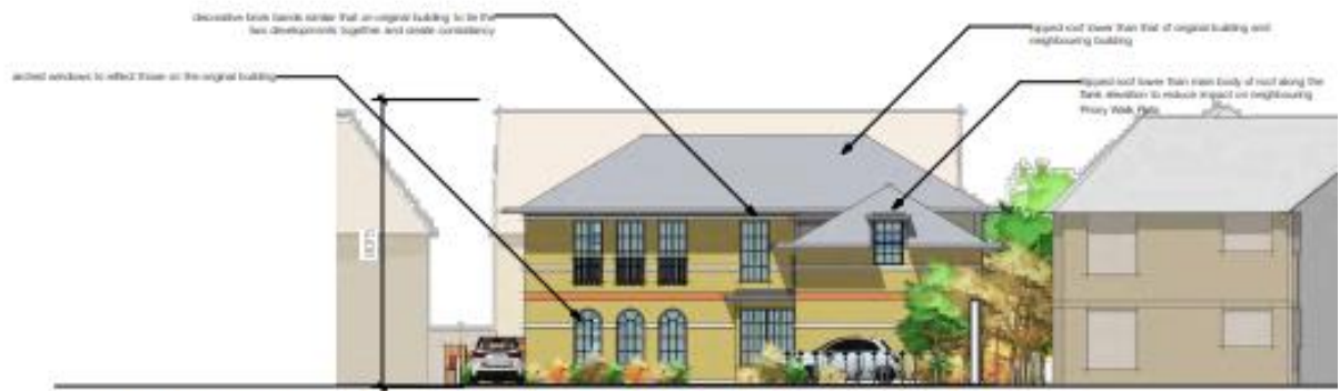
COURTYARD ELEVATION OF NEW BUILDING AS PROPOSED
